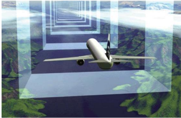
(Fig.4) Precise WAAS Enabled RNP "Highway In The Sky" Illustration
