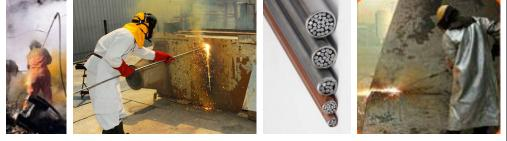
(Left) GZ worker (2<sup>nd</sup> & 3<sup>rd</sup> from left) Demonstration of the pictured thermic lances (exterior is mild steel, all internal rods are steel except for one aluminum rod);<sup>xiii</sup> Notice the iron-oxide plume (Right) www.oxylance.com burning bar demonstration; notice the iron-oxide plume
