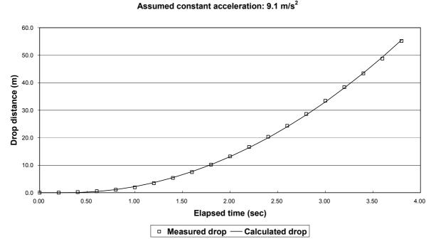
The observed acceleration, 9.1 m/s<sup>2</sup>, if maintained, would bring the roof to the ground in 6.2 seconds, very close to free fall in a vacuum, 6.0 seconds. There is no sign of the slow start that would be expected if collapse was caused by the gradual softening of the steel.
