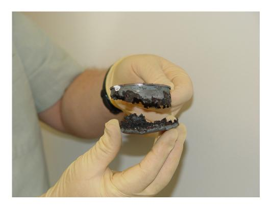
Above: in a fraction of a second, thermate cuts horizontally through a steel cup. Notice the high-temperature corrosion which occurred.
